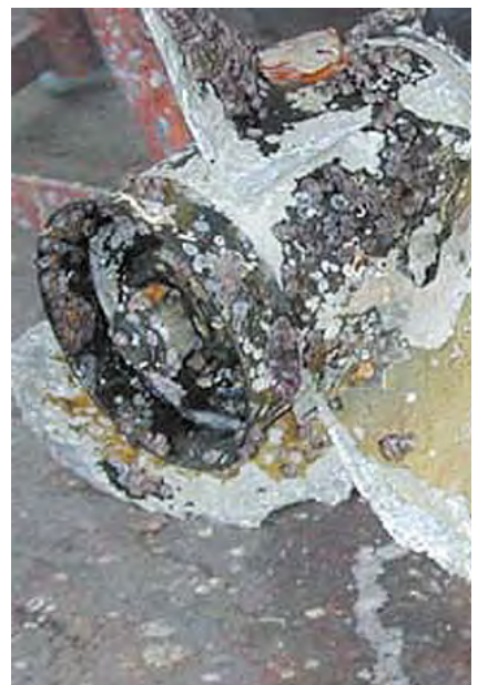
Figure 131.1 Fouling organisms on prop Bob Moffatt
