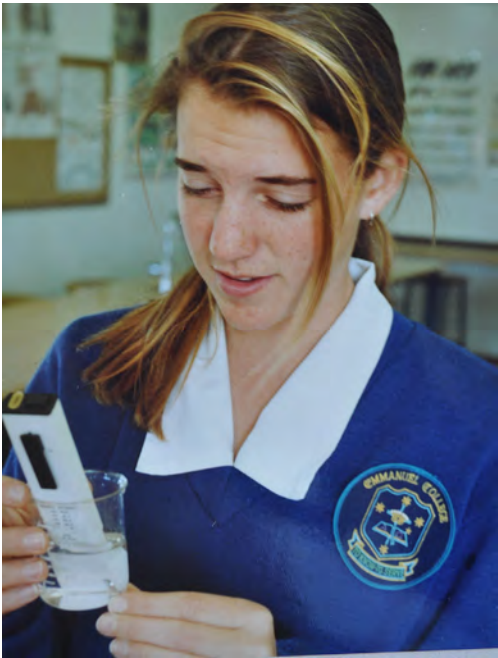
Figure 86.1 Measuring mud salinity with a salinity meter
